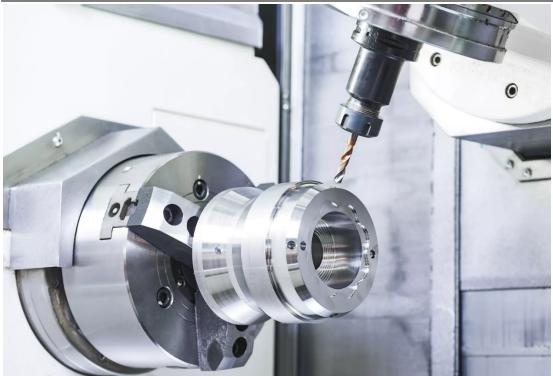
High efficiency and flexibility CNC machining has been commonly recognized as an ideal manufacturing process to make sure high quality in metal parts machining. The whole course of manufacturing process is running on the base of automated machine positioning systems and adjustable fixtures, so it's of greater flexibility to react to production schedules.
