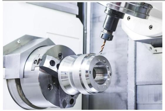
CNC machining has been commonly recognized as an ideal manufacturing process to make sure high quality in metal parts machining. The whole course of manufacturing process is running on the base of automated machine positioning systems and adjustable fixtures, so it's of greater flexibility to react to production schedules.
